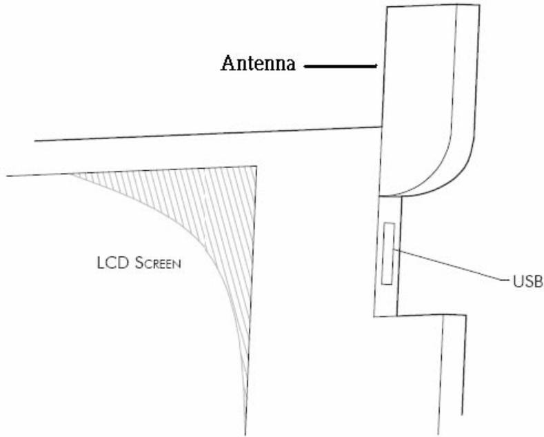
**Figure 2.9: External Antenna**
