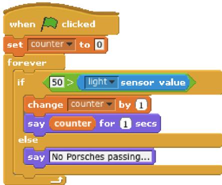
Figure 3: The car counter implementation in Scratch
