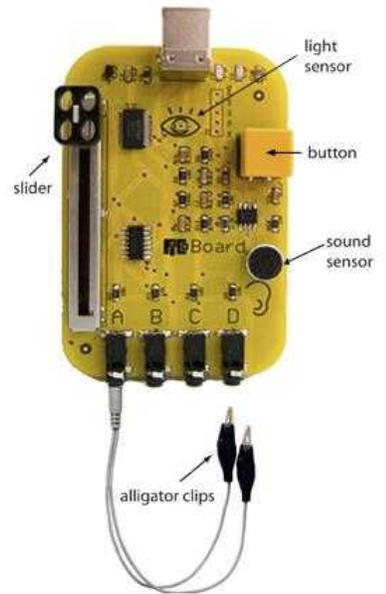
Figure 2: The picoboard for the car counter (picture taken from <http://www.picocricket.com/picoboard.html>)
