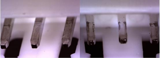
Machines which have experienced vibration and/or thermal cycling, should be disassembled and inspected for signs of fretting corrosion, especially on the battery cable connector. The floating nature of this design should prevent relative motion, and is good practice. Still, a resistance check and visual inspection of connectors from thermal and vibration test machines, will be important to verify the design.
