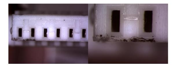
Connectors CN25 and CN26 are identical to CN22. Removing the cables from CN25 and CN26 is straight forward. However, removing the cable from CN22 is made more difficult by the solder bump from a feed through just in front of the female end.
