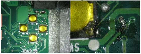
In the battery compartment, one machine had a missing spacer. These are small pads that are apparently attached with adhesive.
