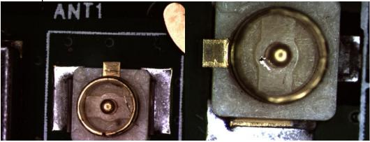
Several connector pairs have mismatched plating types, with gold on one side and tin on the other. And pairs are inconsistent with gold on gold in some machines while tin on gold in others. Gold flash is possible in some that appear tin, but it was not observed. This may be a supply issue but if you are paying for gold, you should get gold.
