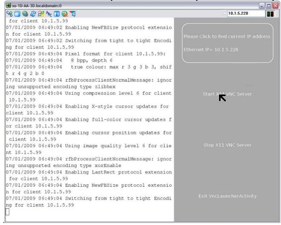
Click "Stop X11 VNC Server" or Exit VNC Launcher Activity, when you want to disconnect XO from your PC. But "Exit VNC Launcher Activity" will close down the Activity. The Stop button will only stop connection and allow you to start the connection anytime.
