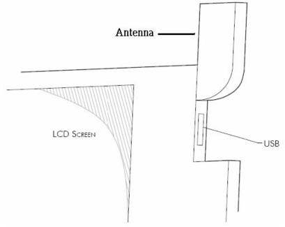
Figure 2.9: External Antenna
